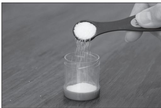
Adding sand in measured increments
