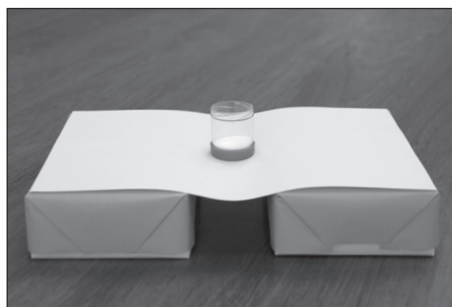
Suspended A4 paper with weight supported
